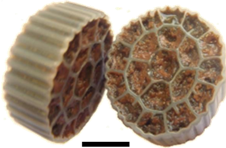
Figure SI 2: Carrier material (Type K3, AnoxKaldnes, Sweden) used in this study. Scale bar 10 mm.
