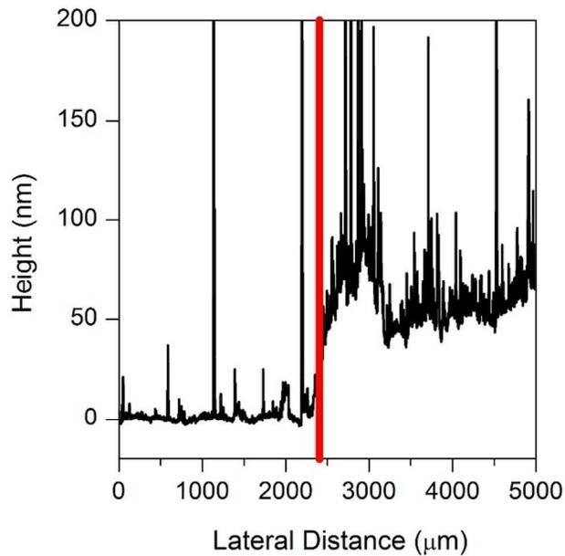
**Figure 2.** Profilometry scan of the RGO electrode. The solid red line indicates the edge of the RGO film. Note both the film height ( $\sim 50$  nm) and the film roughness.
