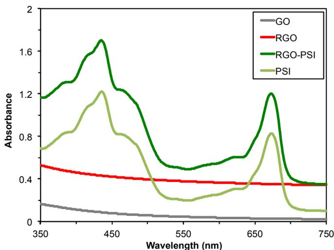
**SFigure 5.** UV-Vis spectra of PSI-modified RGO film (dark green), PSI film on unmodified glass (light green), unmodified RGO film (black), and GO film (red).
