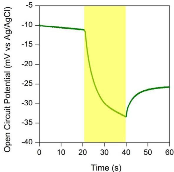
**SFigure 7.** Photovoltage measurement of a PSI modified RGO electrode using 2 mM DCPIP and 100 mM KCL as the electrochemical mediator. The photovoltage was determined by the change in the open circuit potential as the system changed from a dark to an illuminated condition (20-40 s).
