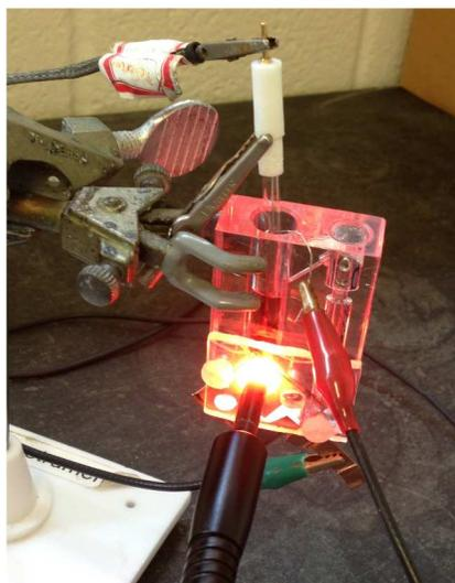
**Figure 6.** Half-cell set-up with the PSI-modified RGO as the active electrode, platinum mesh as the counter electrode, and Ag/AgCl as the reference electrode. The photoelectrode is illuminated directly instead of directing the light through the mediator solution.
