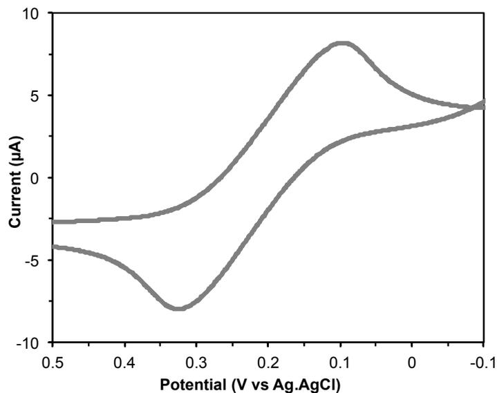
**SFigure 4.** Cyclic Voltammetry of a RGO electrode in 1 mM ferricyanide/1 mM ferrocyanide mediator solution, with 100 mM KCl as the supporting electrolyte, Ag/AgCl as the reference electrode, and platinum mesh as the counter electrode. The scan rate was 1 mV/s.
