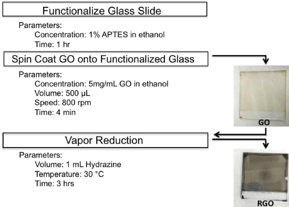
**SFigure 1.** Flow chart summarizing the method for preparing the RGO film and the specific parameters.
