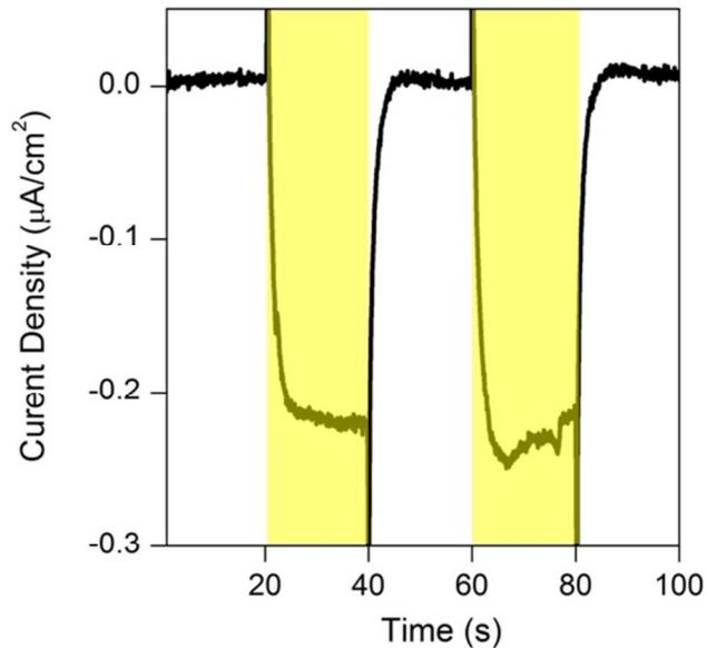
**Figure 8.** Photochronoamperometry of DCPIP using an FTO electrode. The electrochemical mediator consisted of 2 mM DCPIP and 100 mM KCl. The sample was illuminated from 20-40 seconds and 60-80 seconds as indicated by the shaded areas.
