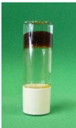
Figure S6: Phase selective gelation of a mixture of water and petrol. In the picture, the fluid liquid aqueous phase is retained by the gelled petrol (inverted flask)
