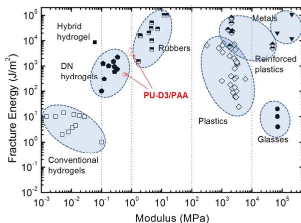
**Figure S2.** Fracture energy of various materials<sup>16,27</sup> vs. their modulus compared with the PU-D3/PAA hydrogels developed here (open circles).
