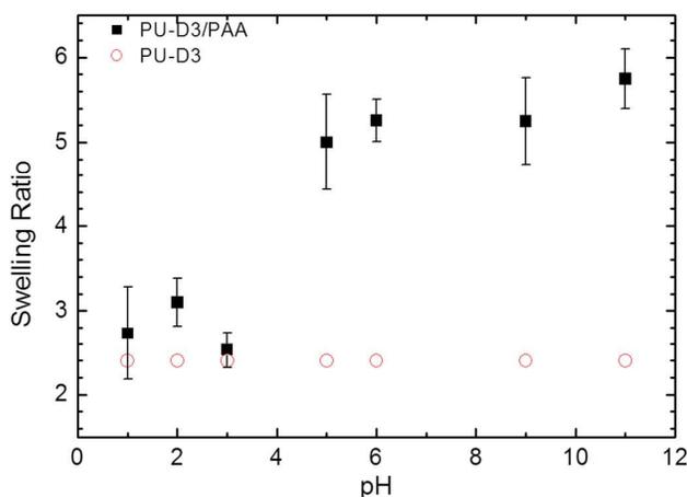
**Figure S1.** Swelling ratio of PU-D3 (open circles) and PU-D3/PAA hydrogels (filled squares) equilibrated at different pHs. Error bars indicate the standard deviation for three measurements.
