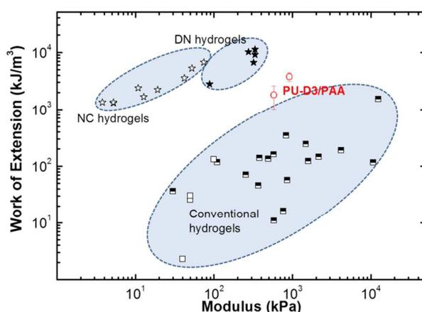
**Figure S4.** Work of extension of various hydrogels<sup>16</sup> and their corresponding modulus compared with the PU-D3/PAA hydrogels equilibrated at pH 2 and pH 6 (open circles). The half-filled squares represent hydrophilic-hydrophobic copolymer hydrogels with lower swelling ratio (see Figure S5) and higher modulus.
