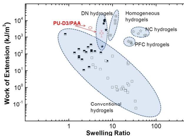
**Figure S5.** Work of extension and swelling ratio of various hydrogels<sup>16</sup> compared with those of PU-D3/PAA hydrogels equilibrated at pH 2 and pH 6 (open circles).
