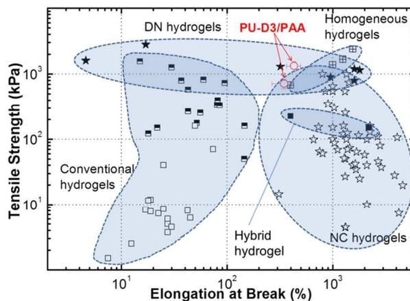
**Figure S3.** Tensile strength of various hydrogels vs. their corresponding elongation at break. Open circles represent the PU-D3/PAA hydrogels developed here and equilibrated at pH 2 and pH 6. The half-filled squares are hydrophilic-hydrophobic copolymer hydrogels used in contact lenses.<sup>16</sup> The filled squares represent the hybrid hydrogels.<sup>27</sup> Other types of hydrogels are as-labelled.
