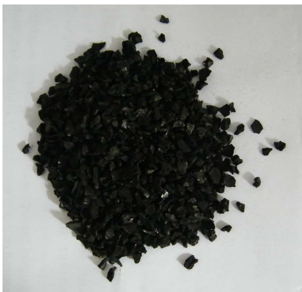
Figure S1. The digital image of the raw coconut shell AC granules.
