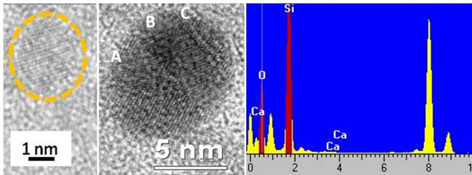
Figure S3. High resolution transmission electron images of SiNCs (left and middle) exhibiting typical fringes of crystalline structure; on the right energy dispersive spectroscopy of the particle in the middle image.
