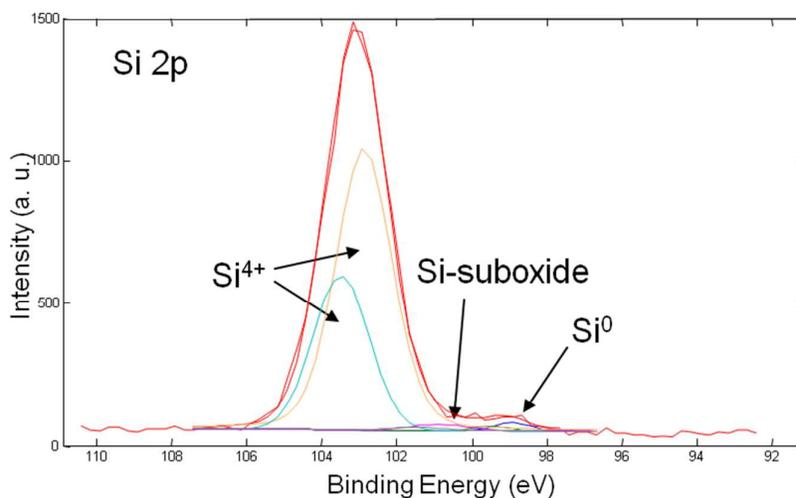
Figure S2. X-ray photoelectron spectrum Si 2p of silicon nanocrystal powder stored in water for about 3 days.
