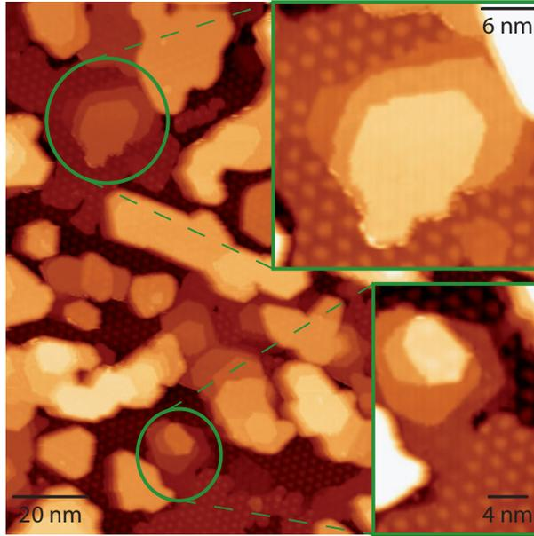
**Figure S1:** Overview STM image of room temperature deposited Au on monolayer graphene/Ru(0001), observed by UHV STM at 77 K ( $V_{sample} = -0.27$  V,  $I = 0.46$  nA). Circles mark islands shown in the close-up views whose terraces are partially or completely flat.
