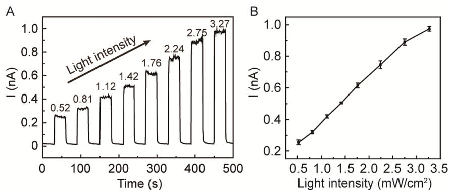
Figure S4. (A) Photocurrent of  $\text{In}_2\text{Se}_3$  flakes as a function of incident light density. (B) The output photocurrent change with incident light density.
