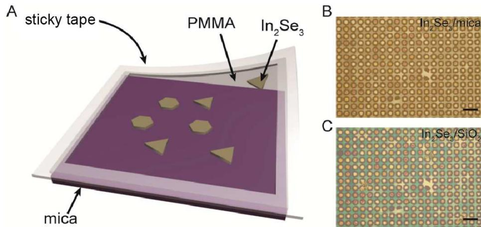
Figure S1. (A) Schematic diagram for the PMMA-mediated transfer technique. (B, C) Optical images of In<sub>2</sub>Se<sub>3</sub> flakes before and after transfer, respectively. Scale bars: 20  $\mu\text{m}$ .
