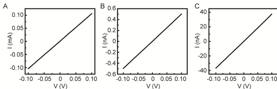
Figure S3. Phase transition of 2D  $\text{In}_2\text{Se}_3$  flakes induced by annealing and electron beam irradiation: (A) Two-probe I-V measurement of an  $\text{In}_2\text{Se}_3$  flake with a superlattice structure; (B) Two-probe I-V curve of the same  $\text{In}_2\text{Se}_3$  flake after annealing; (C) Two-probe I-V curve of the same  $\text{In}_2\text{Se}_3$  after annealing and electron beam irradiation.
