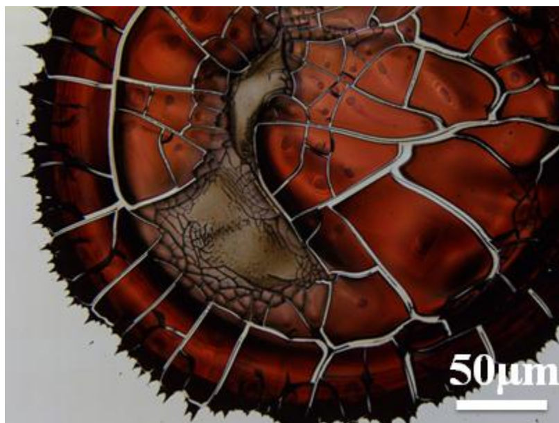
Figure S4. Optical micrograph of PS nanoparticles deposited on the hydrophobic HMDS substrate at 60°C. Highly concentrated ring-like pattern was observed. The large but irregular cracks were also seen due to the evaporation of residual water.
