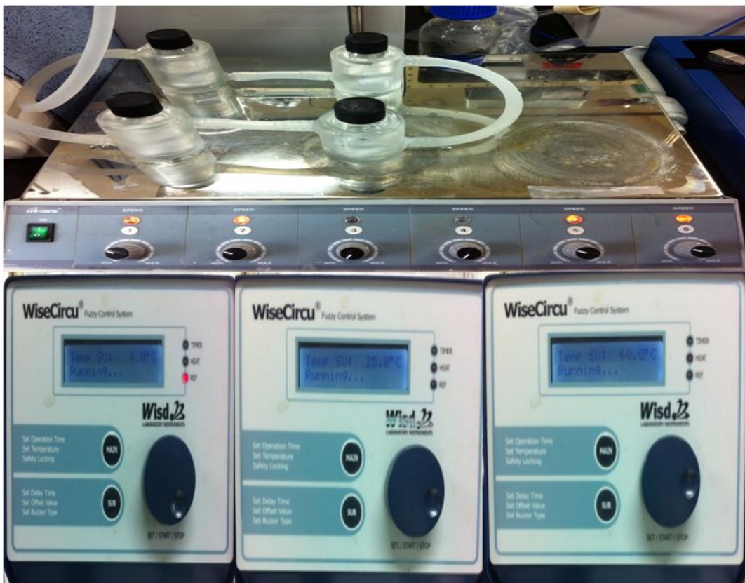
Figure S1. Experimental setup for controlling the metal oxide precursor solution temperature. With this setup, it is possible to synthesize a metal oxide precursor solution and maintain it at a specific temperature.
