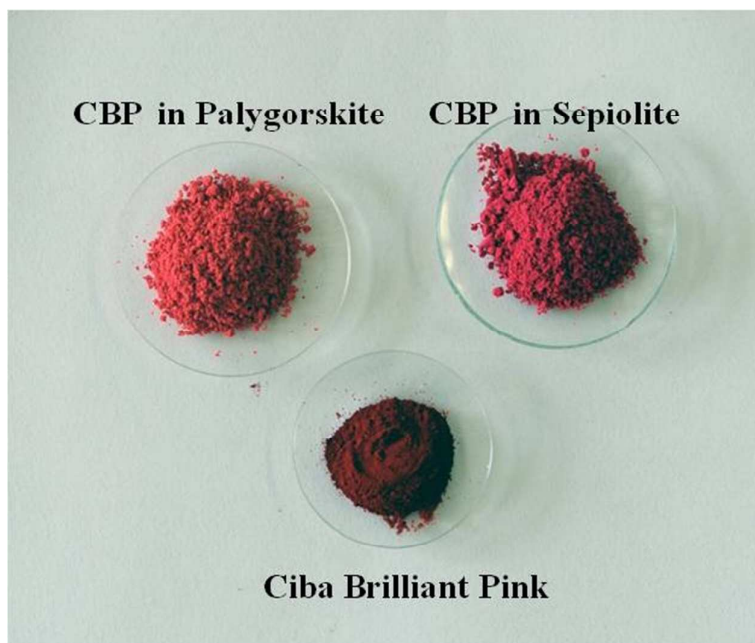
Figure S4. Picture of ciba brilliant pink (down), and ciba brilliant pink mixed with palygorskite (top left) and sepiolite (top right), in a 20% (CBP) w/w proportion.
