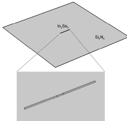
Figure S1 Schematic geometry used in the calculation of the nanowire temperature under a local optical excitation.
