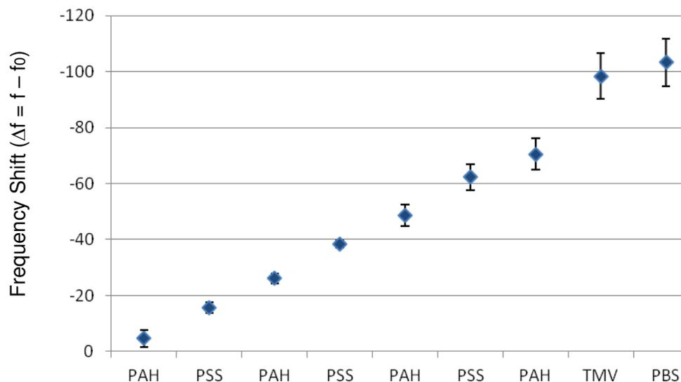
**Supplementary Figure 1.** QCM measurements of PAH/PSS polyelectrolyte membrane with TMV. Each layer of coating decreases the frequency in a linear fashion. TMV coating was followed by incubation in 1x PBS solution for one hour. A slight shift in frequency was observed, likely due to the osmolarity difference between TMV (100 mM K Phos pH 7.0) versus PBS. Error bars denote standard deviation from the mean ( $n = 9$ ) and 3 separate experiments in triplicates.
