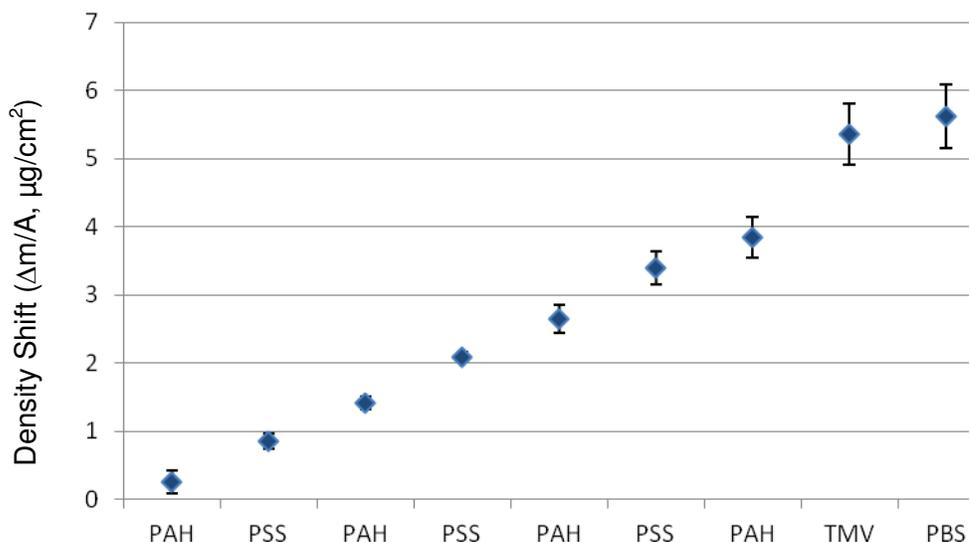
**Supplementary Figure 2.** Mass density shift of polyelectrolyte membrane. A linear mass shift is observed until TMV coating, where the total amount of viral particles averaged  $1.5 \pm 0.3 \mu\text{g}/\text{cm}^2$ . Incubation with PBS solution allowed for slight swelling of the PEM, increasing the density shift by  $0.3 \pm 0.1 \mu\text{g}/\text{cm}^2$ . Error bars denote standard deviation from the mean ( $n = 9$ ) from three separate experiments performed in triplicates.
