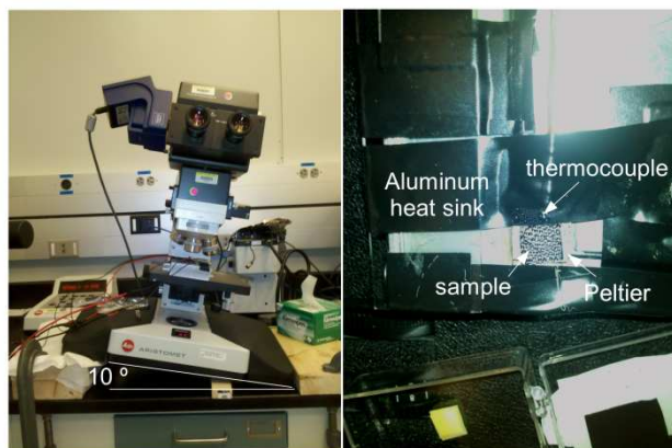
Figure 3. Images of the optical set up used to study liquid marble formation during condensation.
