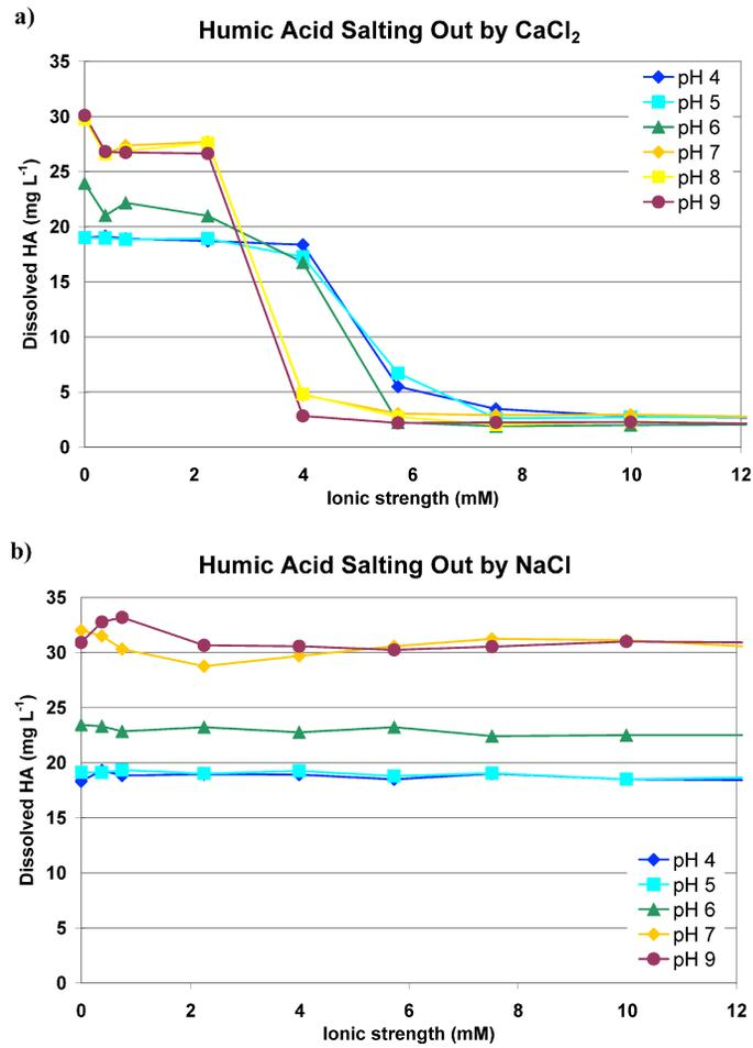
**Figure S.1** Concentration of dissolved ESHA after 24 hr of quiescent salting out by addition of a) CaCl<sub>2</sub> and b) NaCl at equivalent ionic strengths.
