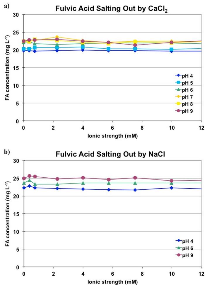
**Figure S.2** Concentration of dissolved ESFA after 24 hr of quiescent salting out by addition of a) CaCl<sub>2</sub> and b) NaCl at equivalent ionic strengths.
