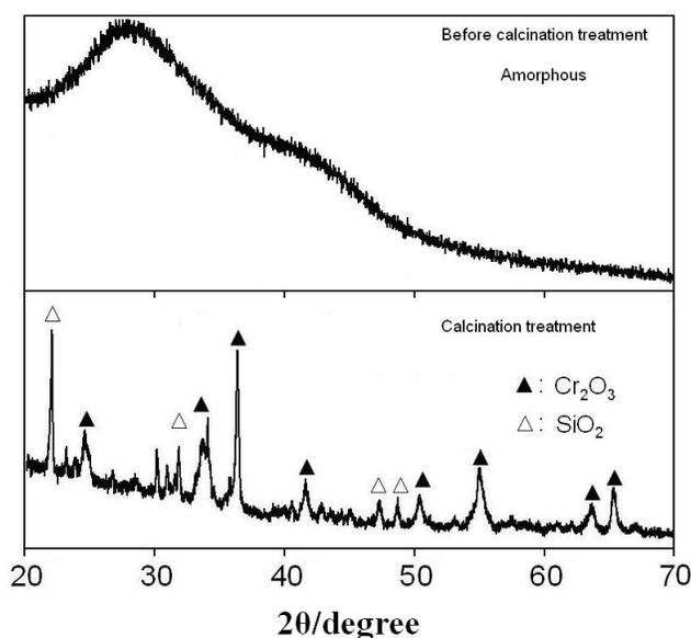
**Figure S4.** XRD data of the Cr-containing bacteria sample before and after calcination. It reveals that the main phase in the solid is Cr<sub>2</sub>O<sub>3</sub> after calcination treatment.
