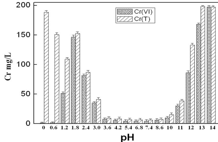
**Figure S1.** The influence of pH on the Cr(VI) reduction and Cr(III) immobilization capability of the cell debris of *O. anthropi*. The initial concentrations of Cr(VI) was 200 mg/L. The cell debris amount was 0.1 g/mL at wet weight and the interacting time was 24 h. The Cr(T) represents total Cr that remained in the supernatant.
