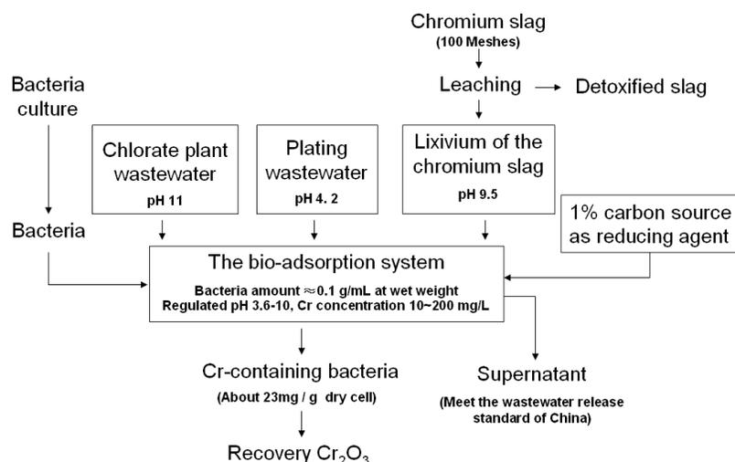
**Figure S3.** The process of pilot-scale treatment with three types Cr(VI)-containing wastewater.
