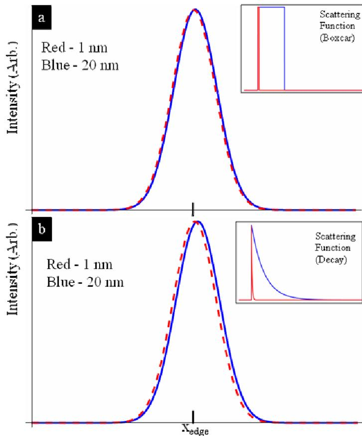
Figure S1: (a) Using the boxcar fit function for the Raman scattering efficiency (this work), we show the convoluted D band intensity for width values of 1 nm (red) and 20 nm (blue), as shown in the inset. The two curves almost overlap; there is a small offset in the position which when corrected for reveals a near-perfect overlap. Increasing the width to  $\sim 50$  nm is required to obtain a curve that is distinguishable upon superposition.
