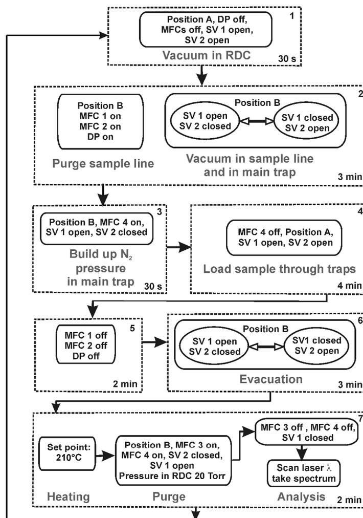
FIGURE S1. Flow chart of the automation sequence for a complete adsorption-desorption and measurement cycle. Each cycle is completed by following 7 steps and the approximate time for completion of each step is indicated. In the chart, DP: diaphragm pump, MFC: mass flow controller, SV: solenoid valve. Positions A and B refer to the two positions of the 12-port valve shown in figure 2 of the paper.
