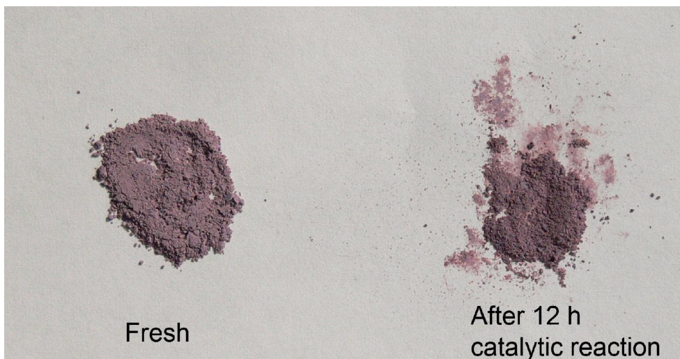
Figure S4. Photographs of the Au/TiO 2 catalyst before and after 12 hours of use.
