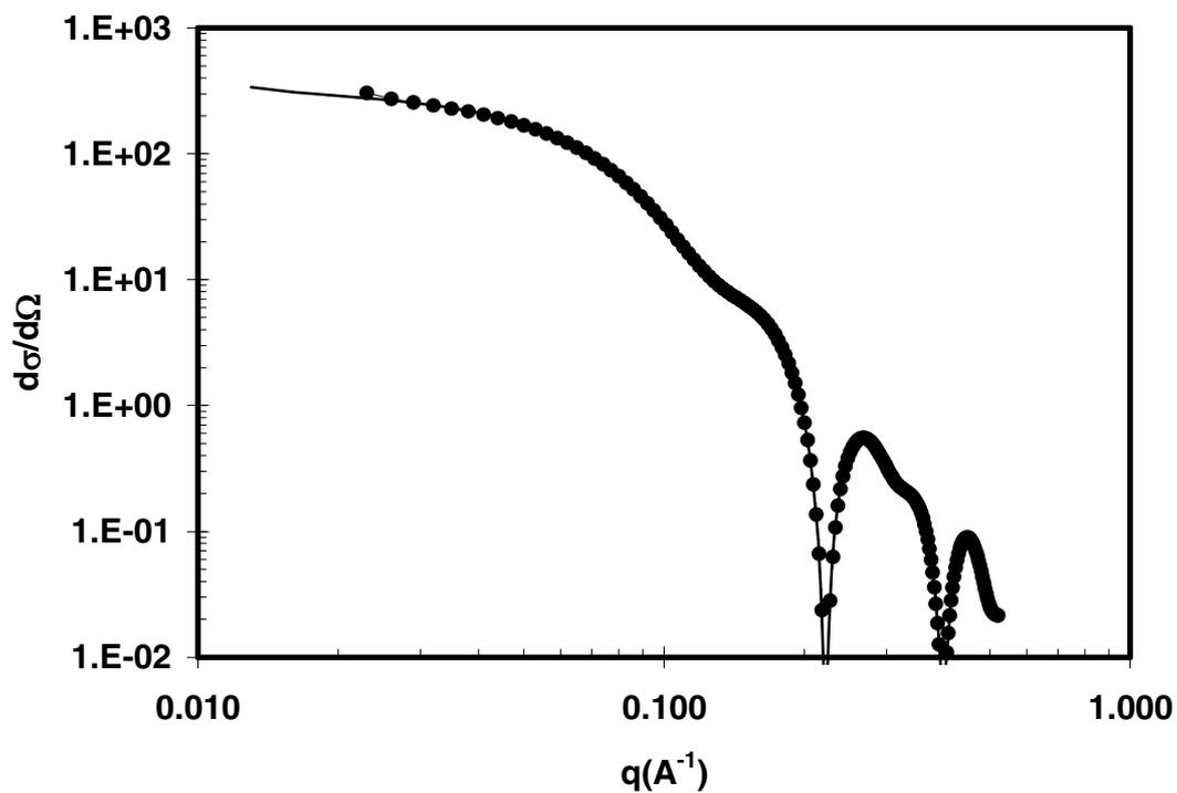
**Figure 2.** Influence of the incident angle of the scattering at two different angles  $0.04^\circ$  (line) and  $0.08^\circ$  (points) when the layer is made of two layers with equal thickness, equal volume fraction but pore radius different by a factor of three.
