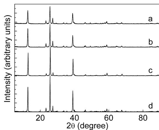
**Figure S1.** XRD patterns of solid products prepared from the 0.9 mol/L molybdenum solution at 170 °C for different time: (a) 1 h, (b) 5h, (c) 20h, and (d) 45h (Figure S1d is identical with Figure 2e).
