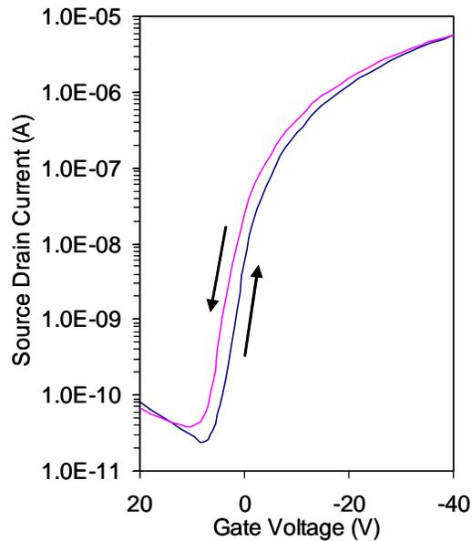
Figure S1. Forward and reverse scans of I-V characteristics at a source-drain voltage of -40 V for a typical OTFT with the dual-layer gate dielectric.
