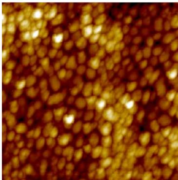
**Figure 3.**  $1 \mu\text{m}$  square height image of Au on a silicon substrate (15 nm height scale).
