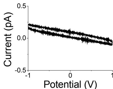
**Figure 2.** Cyclic voltammogram recorded in a solution containing 10 mM  $\text{IrCl}_6^{3-}$  and 0.1 M  $\text{KNO}_3$  at a scan rate of  $20 \text{ mV s}^{-1}$ , using a silicon AFM probe (FESP, L. O. T. –Oriel GmbH & Co.) which had been thermally oxidised for 3 hours by the procedure described above, as the working electrode. An Ag/AgCl reference electrode was employed.
