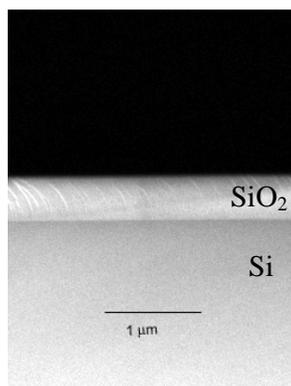
**Figure 1.** FE-SEM cross-section image of a thermally oxidised silicon AFM probe.
