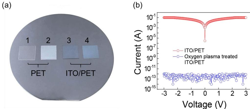
**Figure S5.** (a) Optical image of (1) PET, (2) oxygen plasma treated PET, (3) ITO/PET and (4) oxygen plasma treated ITO/PET films. (b) Current-voltage ( $I$ - $V$ ) characteristics of untreated and oxygen plasma treated ITO/PET films.
