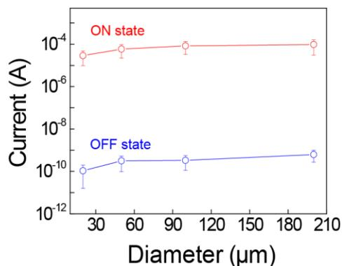
**Figure S6.**  $I_{ON}$  and  $I_{OFF}$  current with respect to the diameter of the top Cu electrode. The error bars represent the standard deviation of 10 working cells.
