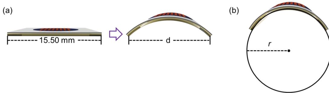
**Figure S2.** (a) Bending method. (b) Estimation of radius of curvature of the flexible Cu/NP WO<sub>3-x</sub>/ITO memory device. The strain (%) was calculated from the equation below.
