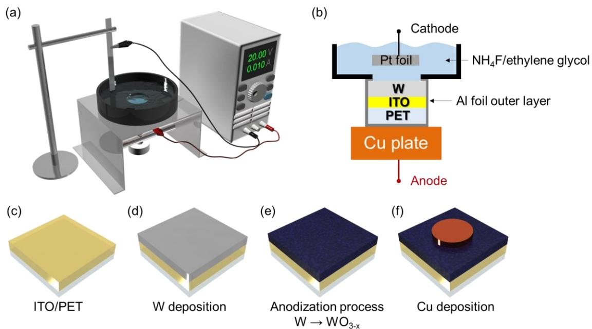
**Figure S4.** (a) Schematic of electrochemical cell used for anodic treatment and (b) sample preparation for anodic treatment. (c) A ~50 nm thick ITO coated film on PET substrate. (d) A 40 nm thick layer of W deposited on the ITO/PET substrate. (e) The W/ITO/PET sample after anodic treatment. (f) A 50 nm thick Cu top electrode deposited through patterned shadow mask on anodic treated sample.
