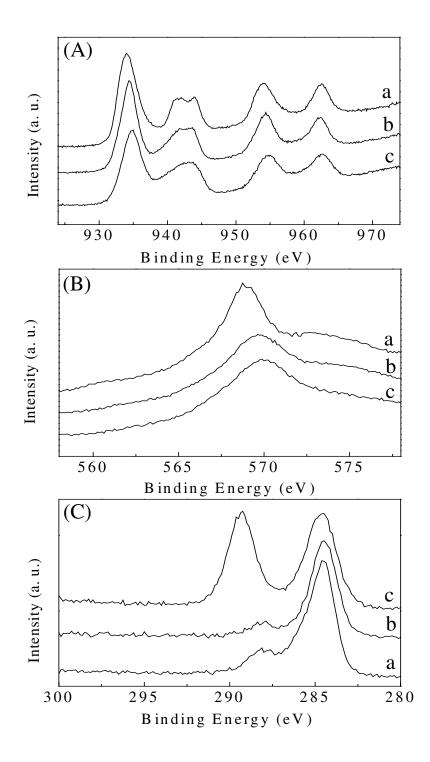
**Figure S2.** (A) Cu 2p XPS spectra; (B) Cu LMM Auger spectra; and (C) C 1s XPS spectra. Curve a: CuO nanosheets/nanowhiskers (from the same sample as used in Figure 2C); Curve b:  $Cu(OH)_2$  nanofibers (from the same sample as used in Figure 2A); and Curve c:  $Cu_2(OH)_2CO_3$  nanorods (from the same sample as used in Figure 2D).
