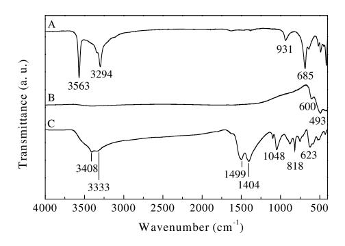
**Figure S1.** FTIR spectra of different samples oxidized from copper foil: (A)  $Cu(OH)_2$  nanofibers (from the same sample as used in Figure 2A); (B) CuO nanosheets/nanowhiskers (from the same sample as used in Figure 2C); and (C)  $Cu_2(OH)_2CO_3$  nanorods (from the same sample as used in Figure 2D).
