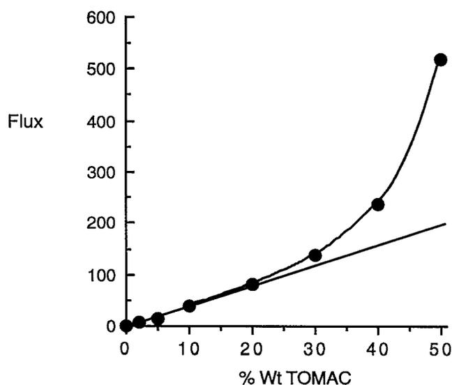
Figure 2. Fructose Flux ( $\text{mol}/\text{m}^2\text{s}$ ) versus % Wt TOMAC for a liquid membrane that also included 2-NPOE. The liquid membrane was supported by a 25  $\mu\text{m}$  thick sheet of Celgard 2500™. Both aqueous phases contained sodium phosphate (60 mL, 100 mM, pH 7.3). The source phase also contained fructose (300 mM).
