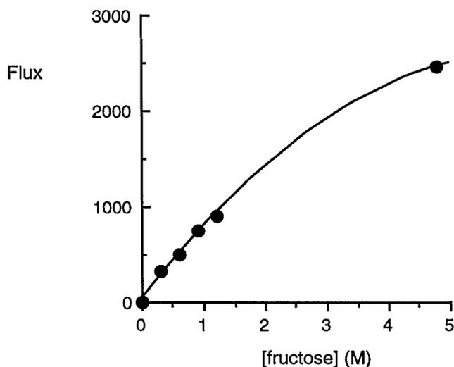
Figure 1. Fructose flux ( $\text{mol}/\text{m}^2\text{s}$ ) as a function of fructose concentration in the source phase. Both aqueous phases contained sodium phosphate (60 mL, 100 mM, pH 7.3). The plasticized membrane (16  $\text{cm}^2$ , 40  $\mu\text{m}$  thick) was manufactured from CTA (0.10 g), TOMAC (0.10 g), 2-NPOE (0.20 g),  $T = 298 \text{ K}$ .
