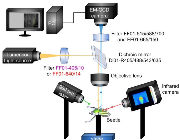
**Figure S1.** Illustration of stereo-microscopy, laser and infrared camera setups. The excitation filter in purple font was used to excite EuDT whereas the excitation filter in red font was used to excite rhodamine 800. The beetle was tethered on top of a stick which was fixed to a metallic stage. The flight muscle was exposed and observed under stereo microscopy. External heating was induced by using a 980 nm laser. The temperature of the muscle was monitored by an infrared camera.
