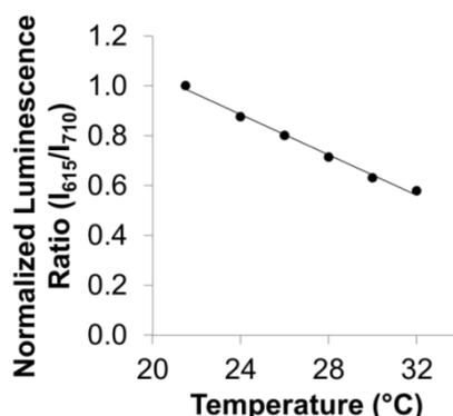
**Figure S4.** The *in vitro* normalized luminescence ratio ( $I_{615}/I_{710}$ ) plotted against the varying temperature, with the absolute luminescence ratio shown in Fig. 1e. The ratio at each temperature was normalized by the ratio at 21.5 °C. The temperature sensitivity, or the gradient of the normalized ratio curve is  $-4.0\%/^{\circ}\text{C}$  relative to 21.5 °C ( $y = -0.040x + 1.86$ ,  $R^2 = 0.99$ ).
