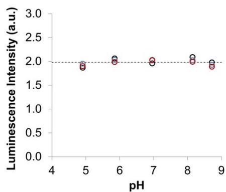
**Figure S9.** Stability of the RNT in MOPS (3-(*N*-morpholino)propanesulfonic acid) buffer with different pH (5-9). The ratio of luminescence intensity of EuDT to that of rhodamine 800 ( $I_{615}/I_{710}$ ) was plotted ( $n = 3$  trials, different colours represent independent trials) against the varied pH of the buffer solution.
