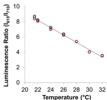
**Figure S7.** Reversibility of the luminescence ratio ( $I_{615}/I_{710}$ ) of the RNT under  $N_2$  saturated solution. The ratio of luminescence intensity of EuDT to that of rhodamine 800 ( $I_{615}/I_{710}$ ) was plotted ( $n = 3$  trials, different colours represent independent trials) plotted against the temperature. The temperature sensitivity or the gradient of the averaged data (black line) is  $-0.48/^\circ\text{C}$  ( $y = -0.48x + 18.83$ ,  $R^2 = 0.99$ ).
