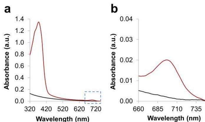
**Figure S3.** UV-vis absorption spectra of the RNT of EuDT and rhodamine 800 embedded PS-MA particles (red lines) and PS-MA particles without dyes (black lines). Graph plotted were the average of multiple measurements ( $n = 5$  measurements). (a) The peak at 370 nm shows the EuDT absorption. The blue rectangular indicates the rhodamine 800 absorption as displayed in the magnified image in (b). (b) The peak at 700 nm shows the absorption of rhodamine 800 in the prepared RNT.
