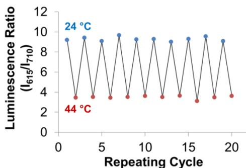
**Figure S6.** The reversibility of the RNT response against the heating-cooling cycle between 24 °C (blue circles) and 44 °C (red circles). For the EuDT channel, the excitation wavelength was 400 nm and the emission was recorded from 550 to 650 nm, while for the rhodamine 800 channel, the excitation wavelength was 635 nm and the emission was recorded from 660 to 750 nm. The luminescence ratio ( $I_{615}/I_{710}$ ) was plotted against the number of heating-cooling cycle.
