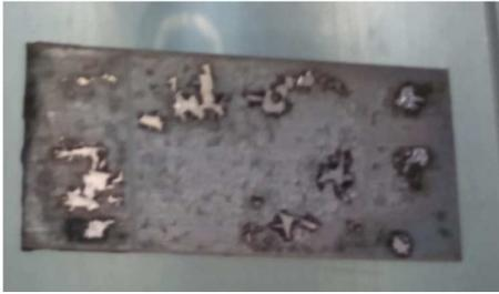
Figure S3. Image of a copper sample after exposure to  $O_2$  plasma at 150 W for 5 minutes. A dark layer of copper oxide was formed after the  $O_2$  plasma. The bright spots observed correspond to the copper substrate where the oxide layer was peeled off. The oxide layer was easily removed because of the poor adhesion with the substrate.
