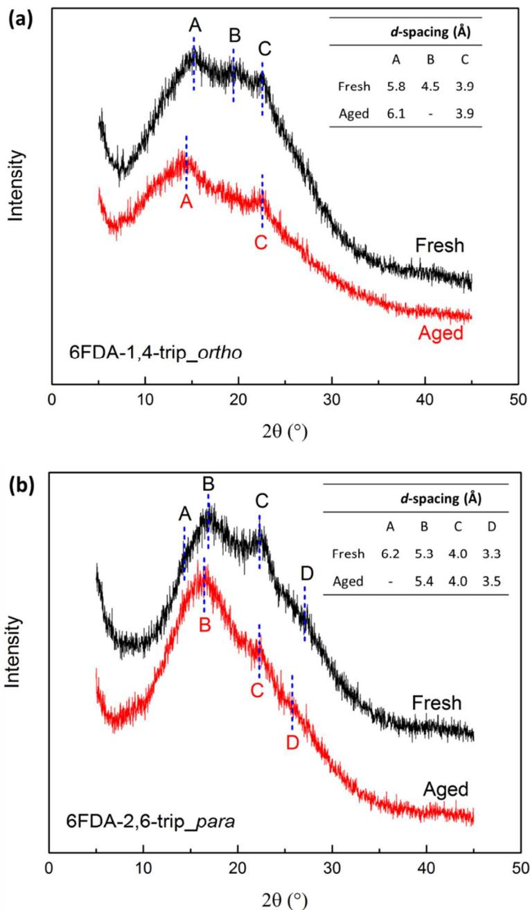
**Figure S6.** Wide-angle X-ray diffraction patterns of (a) fresh and aged (2.5 years) 6FDA-1,4-trip\_ortho films and (b) fresh and aged (5 months) 6FDA-2,6-trip\_para films.
