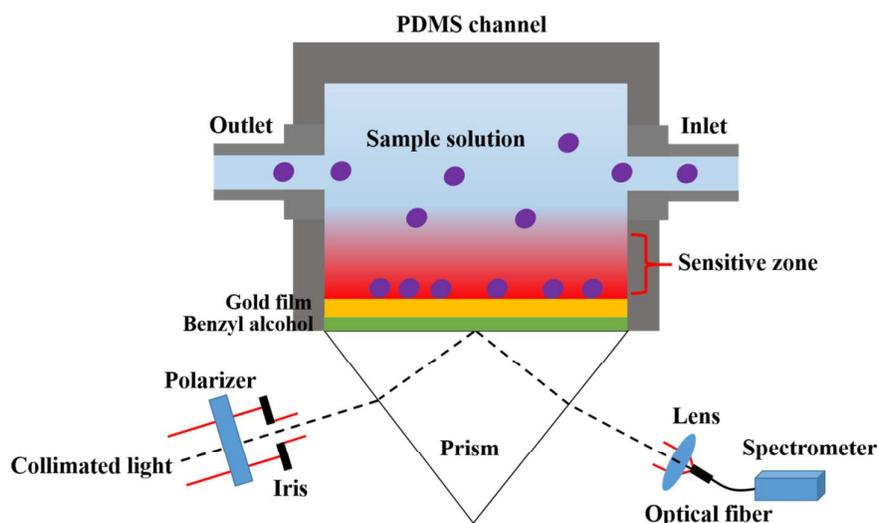
**Figure S1.** Schematic diagram of home-built spectral Surface Plasmon Resonance (SPR)
