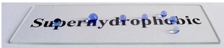
Figure S1. Side-view optical image of blue water droplets spherically positioned on TSS.
