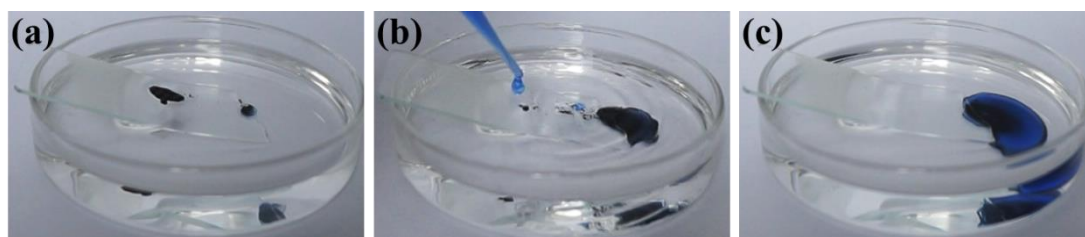
Figure S6. Self-cleaning behaviors of the TSS in petroleum ether after 10 months storage.
