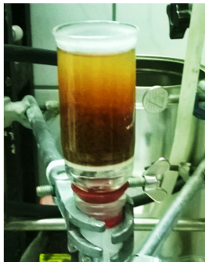
Fig. 3 Filtering crude mixture through a Schott funnel.
