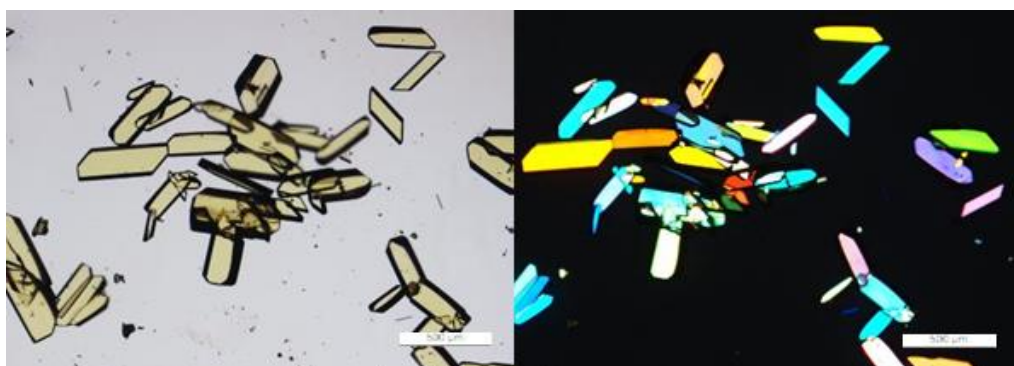
Figure S22. Optical micrographs (scale bar is 500 \mu\text{m} ) of the single crystals grown from 1,3-dimethoxybenzene in bright field mode (left) and between crossed polarisers (right).
