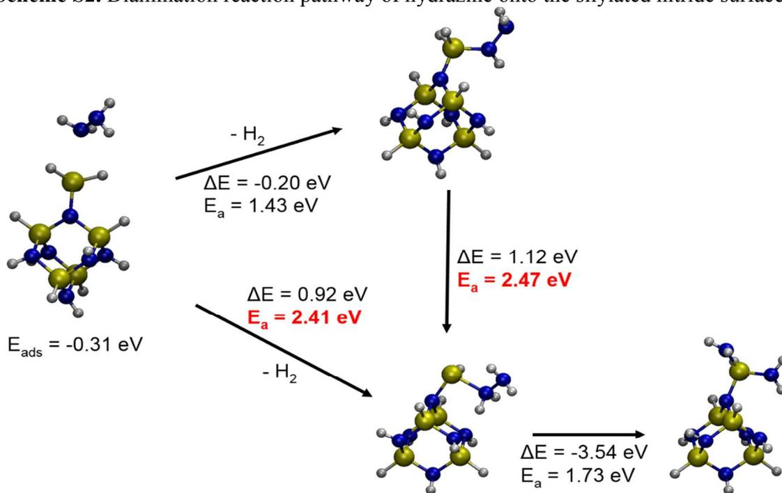
**Scheme S3.** Monoamination reaction pathway of hydrazine onto the aluminum-activated surface.
