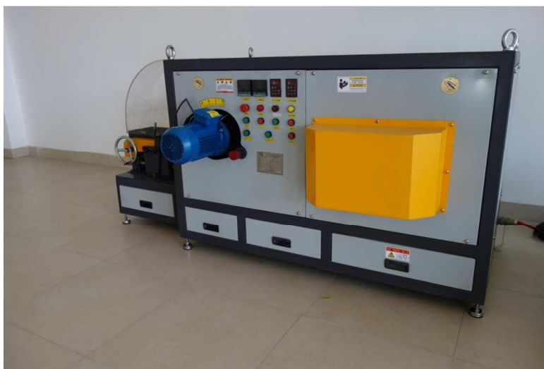
Figure S2. The employed magnetic separator(Company: Fushun Jin Sheng Yu Yi mechanical and electrical equipment manufacturing Co., LTD, China; Capacity: 25 kg/min; Power Rating: 2.75 kW)
