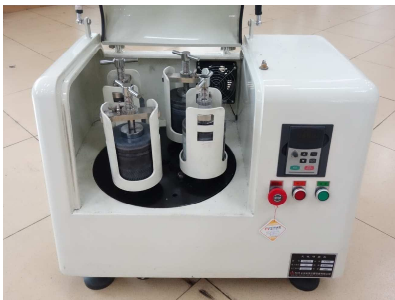
Figure S3. Ball milling machine employed to produce nano- \text{Al}_2\text{O}_3 (Company: Changsha Miqi Instrument Equipment Co., LTD, China ; Capacity: 0.41kg/h ; Power Ratings: 0.75 kW)
