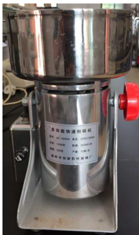
Figure S1. Shearing machine for waste metallic film resistors (Company: Wenling Innovation mechanical equipment manufacturing Co., LTD, China; Capacity: 5 kg/min; Power Rating: 1.3 kW)
