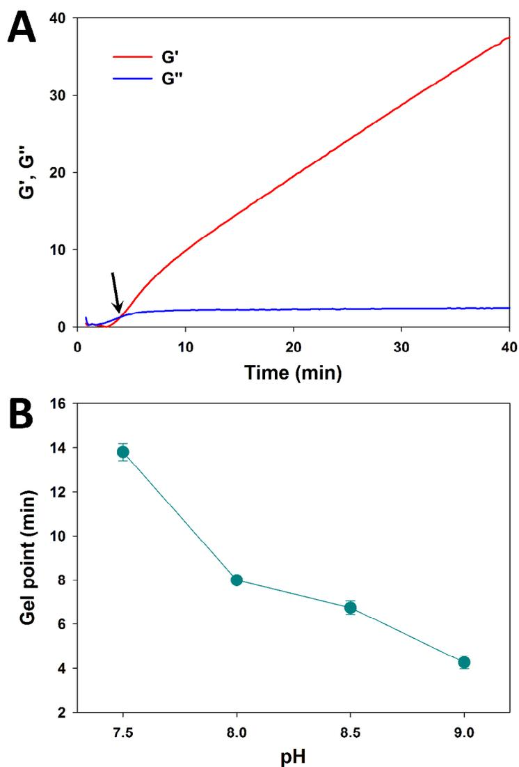
**Figure S9.** (A) Time course of changes in the storage modulus ( $G'$ ) and loss modulus ( $G''$ ) of HA-EGCG hydrogel formed by autoxidation at pH 9.0. The arrow indicates the gel point at which the crossover of  $G'$  and  $G''$  occurs. (B) Gel points of HA-EGCG hydrogels formed by autoxidation at various pH.
