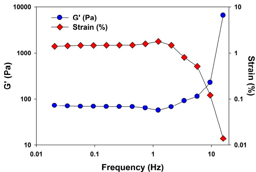
**Figure S8.** Evolution of the storage modulus ( $G'$ ) and strain of HA-EGCG hydrogel as a function of applied frequency of oscillatory shear stress. HA-EGCG hydrogel was formed at the optimized concentrations of HRP ( $0.24 \text{ units mL}^{-1}$ ) and  $\text{H}_2\text{O}_2$  ( $0.76 \text{ mM}$ ).
