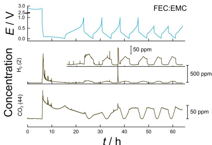
**Figure S4.** Charge-discharge profiles (blue) for the first seven cycles of a Si half-cell with higher loading ( $\sim 0.4 \text{ mg}_{\text{Si}} \text{ cm}^{-2}$ ) using 1 M  $\text{LiPF}_6$  in FEC:EMC with the corresponding background corrected mass signals (brown)  $m/z = 2$  ( $\text{H}_2$ ) and 44 ( $\text{CO}_2$ ).
