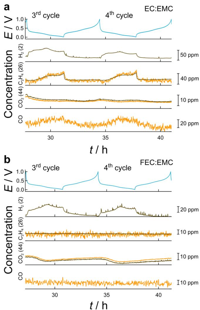
**Figure S3.** Charge-discharge profiles (blue) for the 3rd and 4th cycles of Si half-cells using (a) 1 M LiPF<sub>6</sub> in EC:EMC and (b) FEC:EMC with the corresponding mass signals (brown)  $m/z = 2$  (H<sub>2</sub>), 26 (C<sub>2</sub>H<sub>4</sub>), and 44 (CO<sub>2</sub>), and IR absorption curves (orange) for C<sub>2</sub>H<sub>4</sub>, CO<sub>2</sub>, and CO.
