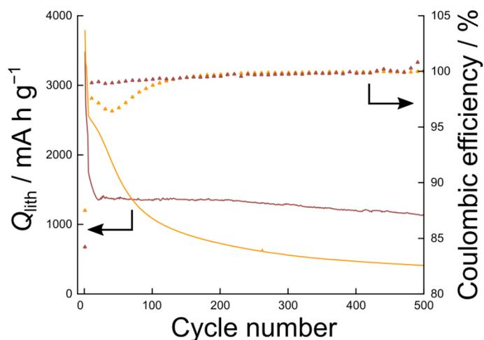
**Figure S1.** Specific lithiation capacities and Coulombic efficiencies for a Si half-cell with higher loading ( $\sim 0.8 \text{ mg}_{\text{Si}} \text{ cm}^{-2}$ ) using 1 M  $\text{LiPF}_6$  in EC:EMC (orange) and FEC:EMC (red).
