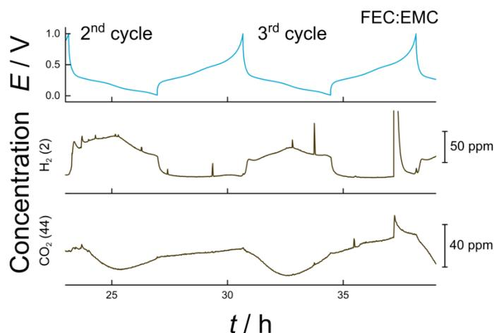
**Figure S5.** Charge-discharge profiles (blue) for the 2nd and 3rd cycles of a Si half-cell with higher loading ( $\sim 0.4 \text{ mg}_{\text{Si}} \text{ cm}^{-2}$ ) using 1 M  $\text{LiPF}_6$  in FEC:EMC with the corresponding background corrected mass signals (brown)  $m/z = 2$  ( $\text{H}_2$ ) and 44 ( $\text{CO}_2$ ).
