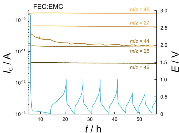
**Figure S2.** Charge-discharge profiles (blue) for the first seven cycles of a Si half-cell using 1 M  $\text{LiPF}_6$  in FEC:EMC with the corresponding ion currents (orange/brown) for the main fragments of  $\text{C}_2\text{H}_3\text{F}$ .
