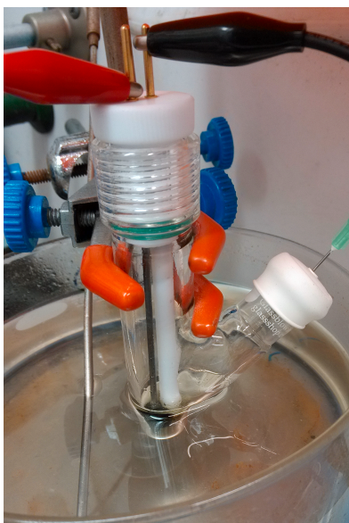
Fig. S1. Setup for the small-scale electrosynthesis of 1,2- trans -dichloroindane (needle on the right is connected to a \text{N}_2 balloon).
