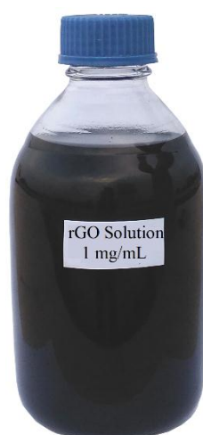
Figure S2. Color image shows large scale (5 L) biosynthesis of rGO using intracellular protein of P. sajor-caju at ambient condition.
