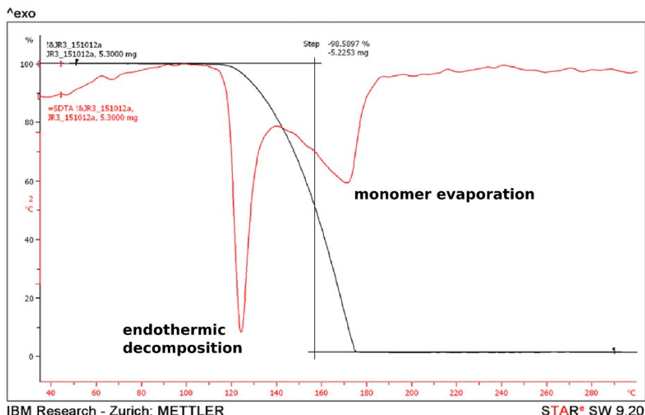
**Figure S2: TGA (black) and DSC (red) traces of the PPA decomposition.**
