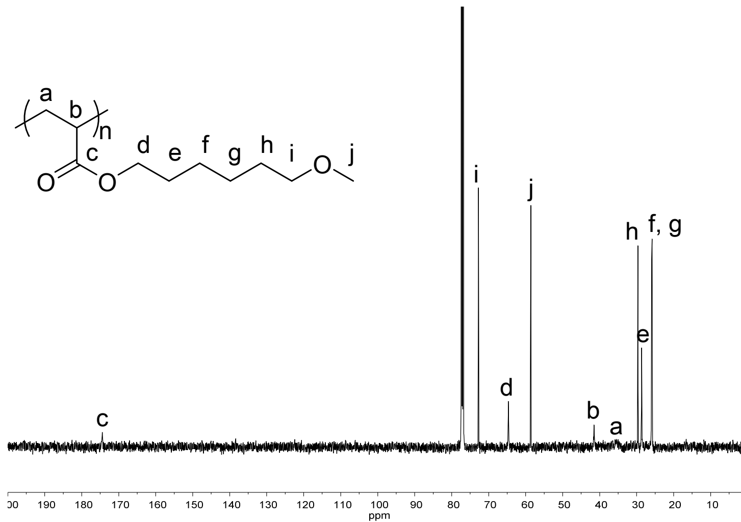
Figure S24. ^{13}\text{C} NMR spectrum of poly(6-methoxyhexyl acrylate) (PMC6A, in \text{CDCl}_3 , 125 MHz).
