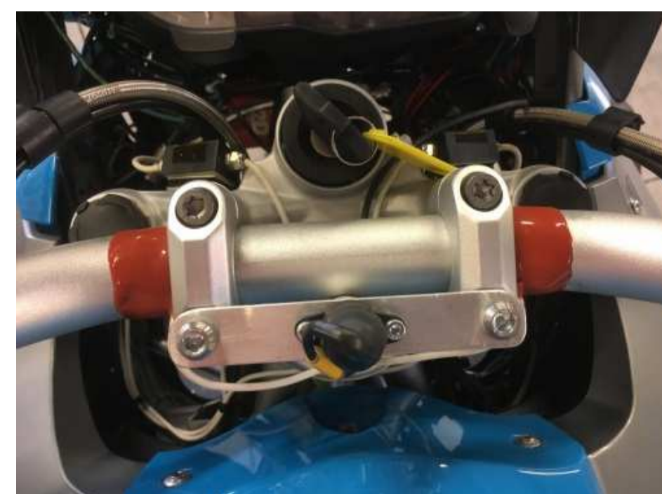
Strain gauges and angle sensor on handlebar
