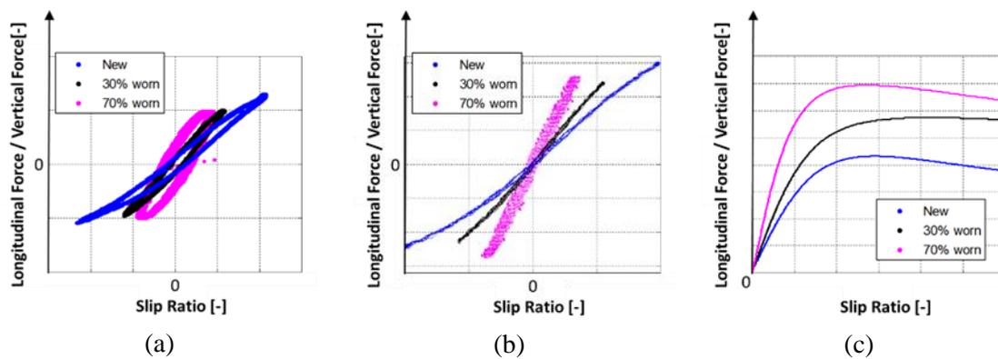
**Figure 9** Flat Track test measurements on tire kinematic-dynamic plane for tire indoor characterization over wear. In particular aimed to characterize: (a): the relaxation length; (b): the longitudinal stiffness; (c): the maximum friction coefficient.
