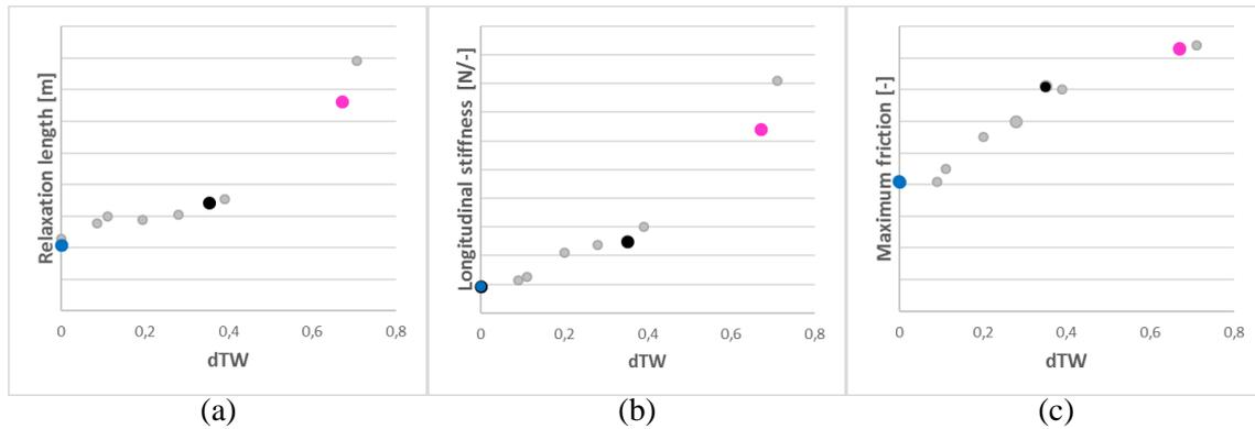
**Figure 10** Flat Track test results for tire indoor characterization: (a): relaxation length characterization over wear; (b): longitudinal stiffness characterization over wear; (c): maximum friction coefficient characterization over wear. Colored dots refer to the tests shown in Figure 9. Gray dots refer to all the other available tests.
