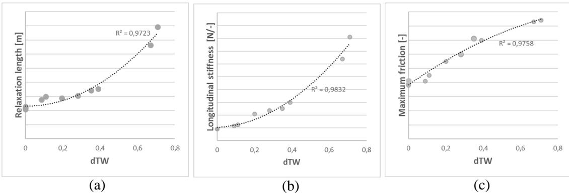
**Figure 12** Tests results for tire indoor characterization: (a): relaxation length characterization over wear; (b): longitudinal stiffness characterization over wear; (c): maximum friction coefficient characterization over wear. Gray dots refer to all the other available tests, dashed line refers to the trendline and  $R^2$  is the trendline correlation coefficient.
