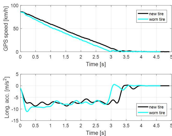
**Figure 5** Experimental test: longitudinal brake maneuver from 80 km/h. In the upper part the speed time history, in the bottom part the longitudinal acceleration time history. In black the signal measured with the new tire, in light blue the ones measured with the worn tire. The worn tire reached higher values of deceleration thus obtaining lower braking distance.
