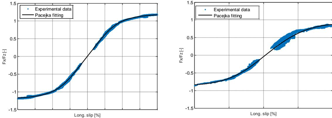
**Figure 11** Experimental data and tire characteristic curves obtained from the fitting procedure: (left side) front tire; (right side) rear tire. Black line refers to the fitting curve using equation (eq. 3).
