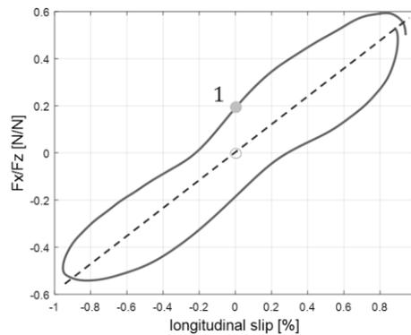
**Figure 8** Indoor test for tire relaxation length characterization: hysteresis cycle between slippage and force.
