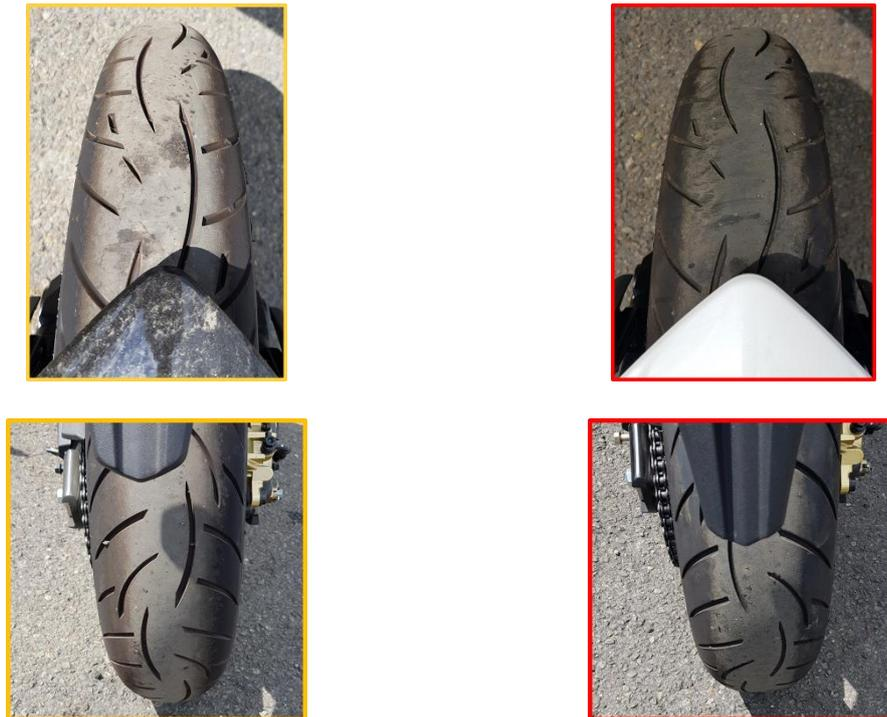
**Figure 3** Experimental test: tires used during the test. New – left side with yellow box, and about 70% worn – right side with red box, conditions. Front tire on first row and rear tire on second row.
