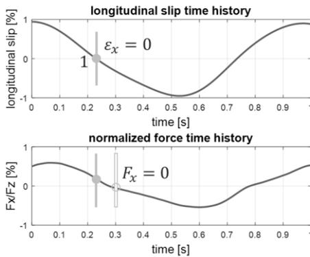
**Figure 7** Indoor test for tire relaxation length characterization: input slip ratio time history and resulting longitudinal force  $F_x$ .
