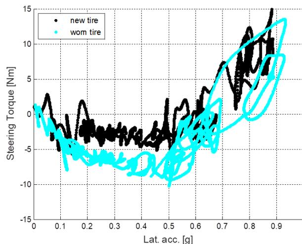
**Figure 4** Experimental test: steering torque variation as function of lateral acceleration. In black the trend for the new tire, in light blue the trend for the worn tire. The steering torque is initially negative, thus directed outbound for both the conditions, but the worn tire has an higher absolute value of the outbound torque.
