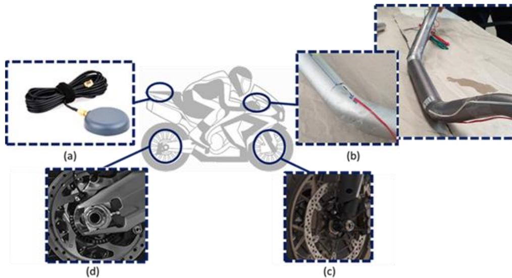
**Figure 1** Motorcycle instrumentation, from top left to bottom right in clockwise direction: (a) high performance GPS for speed and acceleration measurements; (b) strain gauges for steering torque measurement; (c) and (d) respectively front and rear encoders for wheels speed measurements.
