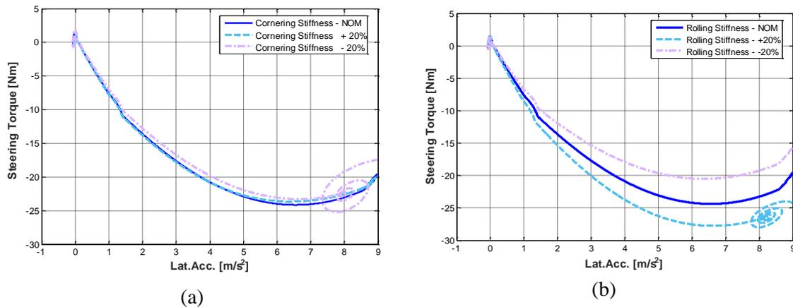
**Figure 6** Steering torque vs. lateral acceleration recorded during a simulated steering pad maneuver with fixed path radius; (a): steering torque variation by changing the cornering stiffness; (b): steering torque variation by changing the rolling stiffness.
