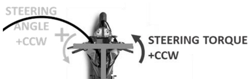
**Figure 2** Experimental test: sign convention for the steering torque measurement. Positive torque when applied in counterclockwise direction, negative torque when applied in clockwise direction.
