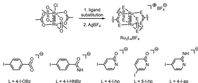
**Figure 2.** Five  $\text{Ru}_2\text{L}_4\text{BF}_4$  complexes were prepared by a two-step procedure of ligand substitution and anion exchange. These complexes feature carboxylate ( $\text{L} = 4\text{-I-OBz}$ ), amidate ( $\text{L} = 4\text{-I-HNBz}$ ), 2-oxyppyridinate ( $\text{L} = 4\text{-I-hp}$  or  $5\text{-I-hp}$ ), and 2-aminopyridinate ( $\text{L} = 4\text{-I-ap}$ ) as the primary coordination spheres, respectively.
