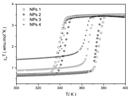
**Figure 3.** Comparison of the thermal variation of the  $\chi_M T$  product for the different hybrid [Fe(Htrz)<sub>2</sub>(trz)](BF<sub>4</sub>)@SiO<sub>2</sub> NPs **1-4** after several heating–cooling modes.
