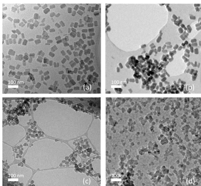
**Figure 1.** HR-TEM images of NPs **1** (a), **2** (b), **3** (c) and **4** (d), deposited by drop casting on holey carbon film in (a) and (c), whereas a lacey carbon film was used in (b) and (c).
