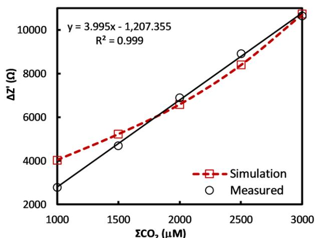
**Fig. 5** TCO<sub>2</sub> calibration for 200  $\mu\text{L}$  sample and receive chambers and 20 min diffusion (0.9 mm gap, 100 mV rms, 0V DC, 100 kHz). The theoretical calibration curve (red) is estimated using a cell constant value of 2100, obtained from 2D finite element simulation of the conductivity cell.
