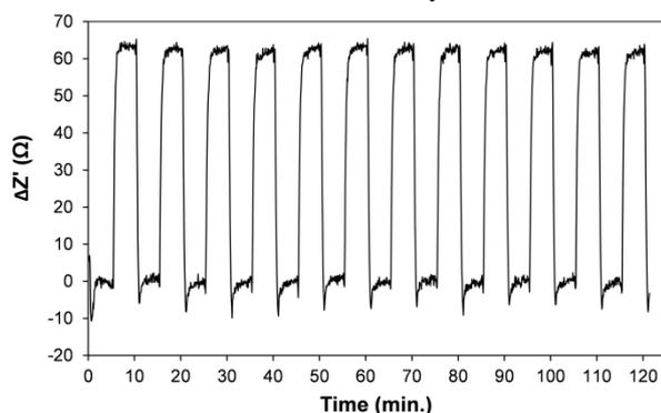
**Fig. 4** Repeatability data for switching between two fluids with a conductivity difference of 1% ( $139.9 \text{ mS m}^{-1}$  and  $141.3 \text{ mS m}^{-1}$ )
