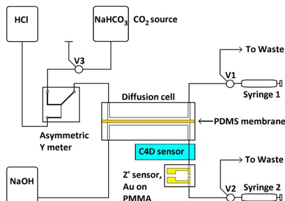
**Fig. 2.** Schematic diagram of negative pressure system for Z' and C4D measurements of TCO<sub>2</sub>. The temperature stabilised water bath is omitted for clarity. The 3-port valves are labelled V1 – V3.
