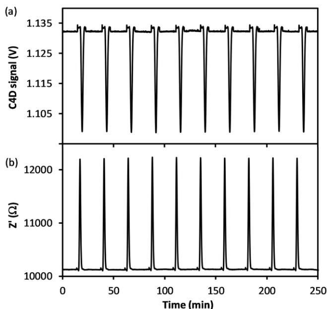
**Fig. 6** (a) C4D peak sequence sample with 2000  $\mu\text{M}$  TCO<sub>2</sub> solution, a 100  $\mu\text{L}$  channel and diffusion time of 15 min, (b) Z' peak sequence sample under same conditions. The conductivity cell interelectrode gap was 0.9 mm.
