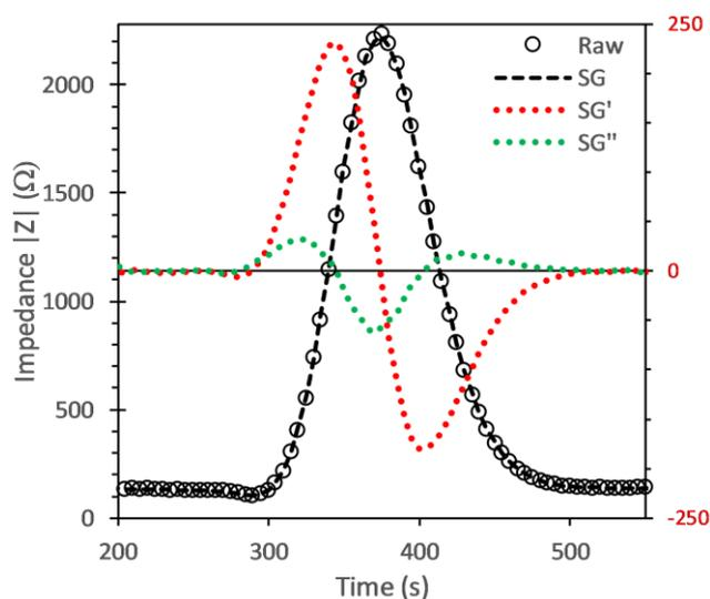
Fig. 8 Elution peak raw data to which a Savitzky-Golay smoothing function is applied (SG). The generated 1<sup>st</sup> (SG') and 2<sup>nd</sup> (SG'') derivatives are used to determine start and end points, along with peak position.
