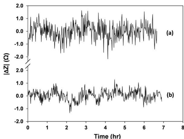
**Fig. 3** Time variation in  $\Delta Z'$  after drift correction, for (a) KCl solution ( $141.3 \text{ mS m}^{-1}$ ) and (b)  $9.1 \text{ mM NaOH}$  solution ( $\sim 220 \text{ mS m}^{-1}$ ).
