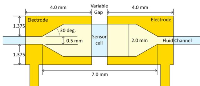
Fig. 1 Electrode pair and sensor cell schematic.
