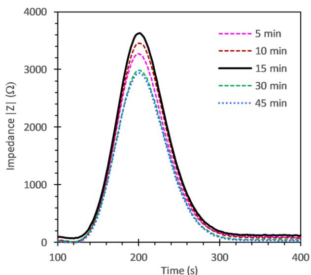
Fig. 7 Elution peak characteristics for diffusion times up to 45 min, with 7 mM NaOH receiving solution.
