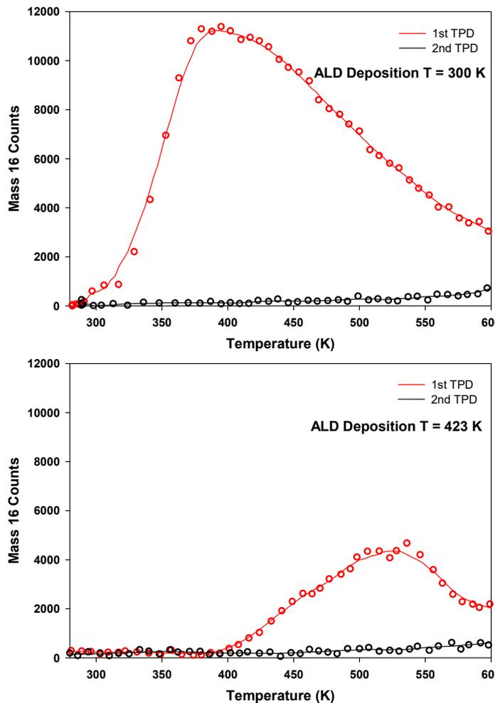
**Fig. S4.** Sequential thermal desorption spectra of mass 16 from 1 ALD/Pt<sub>24</sub>/SiO<sub>2</sub>/Si, with ALD deposited at 300 K (top) and 423 K (bottom).
