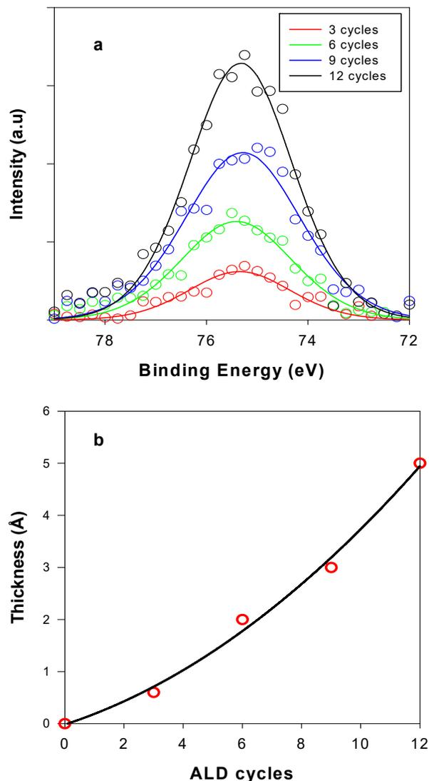
**Fig. 1.** The growth rate calibration of alumina ALD on a clean silica substrate at the surface temperature of 423 K. (a) XP spectra of Al 2p (b) Calculated thickness of Al<sub>2</sub>O<sub>3</sub> as a function of ALD cycles.
