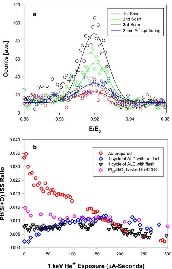
Fig. 4. Pt ISS results for (a) three consecutive high flux ISS scans and a final scan after 2 min of 1 keV  $\text{Ar}^+$  sputtering on the sample 1ALD/ $\text{Pt}_{24}/\text{SiO}_2/\text{Si}$ , where ALD was performed at the substrate temperature of 423 K. (b) Normalized Pt ISS intensity for  $\text{Pt}_{24}/\text{SiO}_2/\text{Si}$  (red), samples with 1 cycle of ALD overcoat with (black) or without (blue) flash post-treatment, and a sample annealed at 423 K in vacuum (pink).
