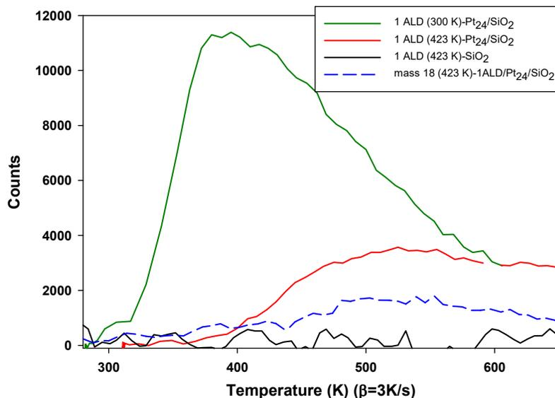
**Fig. 6.** Mass 16 TPD following a single alumina ALD cycle on Pt<sub>24</sub>/SiO<sub>2</sub>/Si at either 300 K (green) or 423 K (red), and on SiO<sub>2</sub>/Si at 423 K (blue). Mass 18 desorption from 423 K 1 ALD-Pt<sub>24</sub>/SiO<sub>2</sub>.
