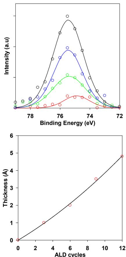
**Fig. S1.** The growth rate calibration of alumina ALD on clean SiO<sub>2</sub>/Si (100) at the surface temperature of 423 K. Dose pressures for H<sub>2</sub>O and TMA were increased to  $5 \times 10^{-5}$  Torr. Calculated thickness of Al<sub>2</sub>O<sub>3</sub> is shown as a function of ALD cycles.
