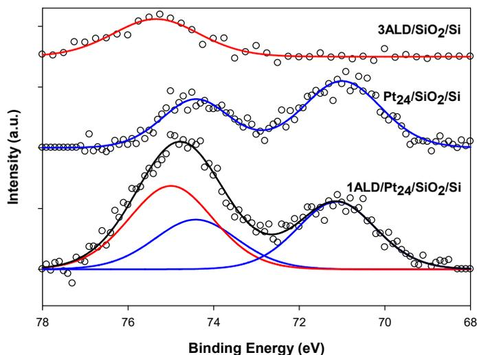
**Fig. 2.** XPS of the Pt 4f and Al 2p region. Top: spectrum for a SiO<sub>2</sub>/Si substrate after three 3 ALD cycles (423 K). Middle: Spectrum of as-deposited Pt<sub>24</sub>/SiO<sub>2</sub>/Si. Bottom: Spectrum for Pt<sub>24</sub>/SiO<sub>2</sub>/Si after one ALD cycle (423 K), with fits showing contributions from Al 2p (red) and Pt 4f (blue).
