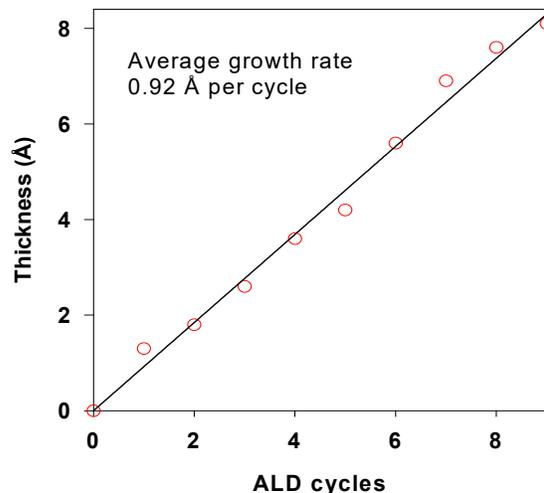
**Fig. S2.** The growth rate calibration of alumina ALD on clean  $\text{SiO}_2/\text{Si}$  (100) at the surface temperature of 300 K. Calculated thickness of  $\text{Al}_2\text{O}_3$  is shown as a function of ALD cycles.
