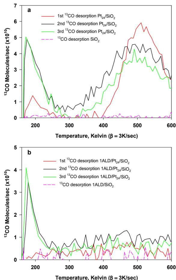
**Fig. 5.** (a) <sup>13</sup>CO desorption from Pt<sub>24</sub>/SiO<sub>2</sub>/Si for three consecutive CO TPDs (solid), and a blank SiO<sub>2</sub>/Si sample (dashed), after 10 L <sup>13</sup>CO exposure at 180 K. (b) <sup>13</sup>CO desorbing from Pt<sub>24</sub>/SiO<sub>2</sub>/Si with 1 cycle of ALD overcoat for three consecutive CO TPDs (solid) and a blank SiO<sub>2</sub>/Si sample with 1 cycle of ALD overcoat (dashed).
