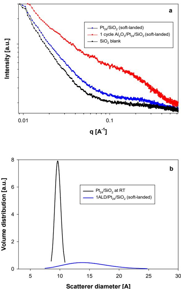
**Fig. 3.** GISAXS for soft-landed Pt<sub>24</sub>/SiO<sub>2</sub>/Si transferred in air, an ALD overcoated sample, and a clean blank SiO<sub>2</sub>/Si sample. (a) Raw GISAXS scattering data (b) Fitted size distributions extracted by fitting the scattering data as in (a) for soft-landed Pt<sub>24</sub>/SiO<sub>2</sub>/Si, as well as soft-landed Pt<sub>24</sub>/SiO<sub>2</sub>/Si with 1 cycle of Al<sub>2</sub>O<sub>3</sub> ALD overcoat.
