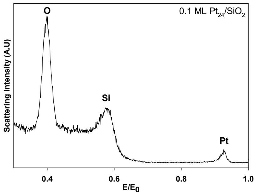
**Fig. S3.** Full energy range ISS scan of as-deposited Pt<sub>24</sub>/SiO<sub>2</sub>.
