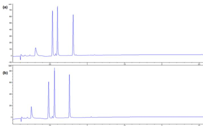
Figure 3: No significant change in chromatographic performance after the installation of the in-line filter, and back-flush. (a) Sample prior to installation.(b) Sample post installation.
