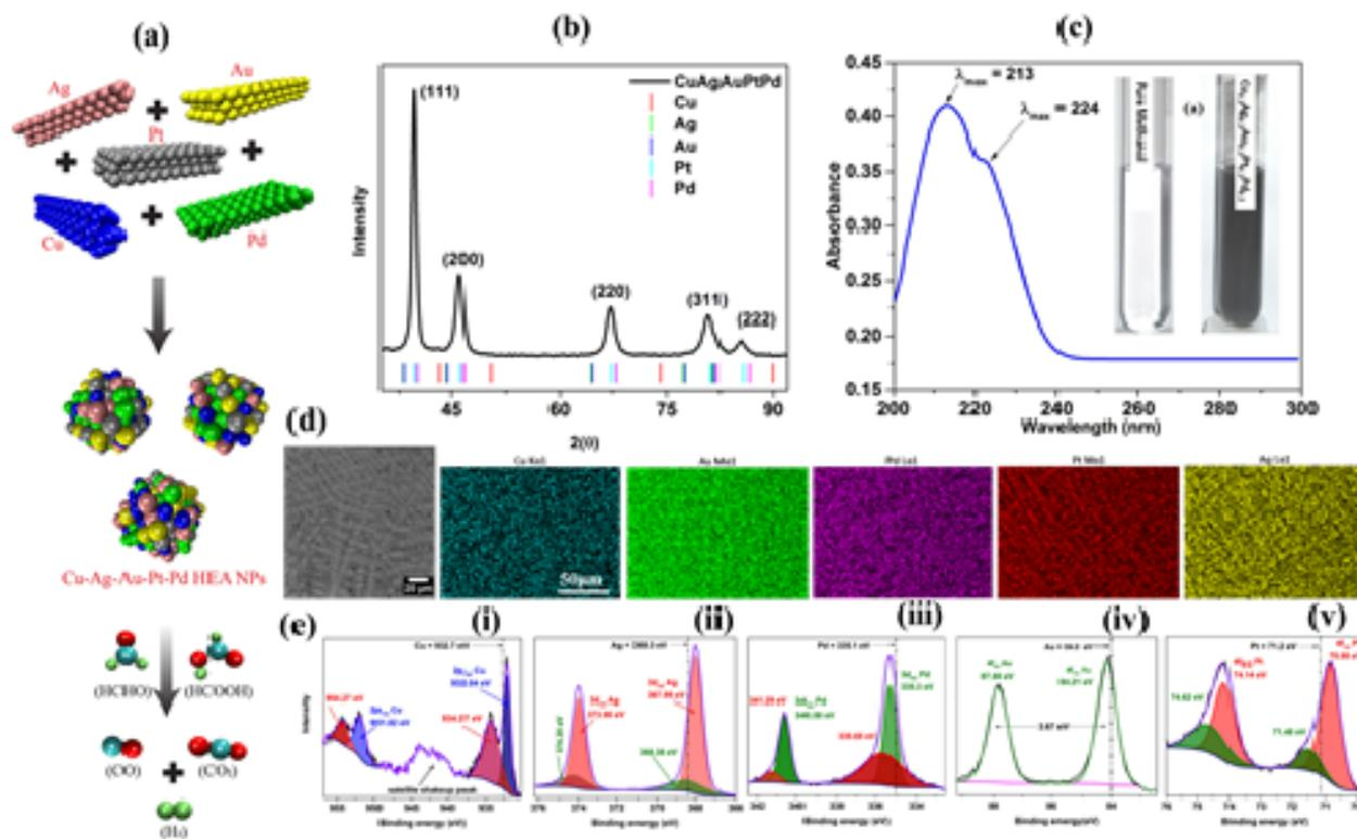
**Figure.1: Materials Characterization of HEAs:** (a) Schematics of HEA nanoparticle preparation and its activity; (b) X-ray diffraction pattern of Cu-Ag-Au-Pt-Pd (ingot) as well as nanoparticles (inset shows (111) peak broadening); (c) UV absorbance spectra of nanoparticles dispersed in pure methanol; (d) BSE image of ingot surface (e) SEM-EDAX elemental mapping of ingot surface; (f) X-ray photoelectron spectroscopy spectra of prepared Cu-Ag-Au-Pt-Pd nanoparticles.
