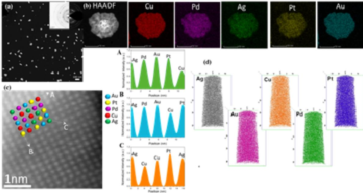
**Figure.2: Composition analysis of HEAs:** (a) Low magnification darkfield image with large number of particles, inset shows selected area diffraction covering several particles, revealing 111, 200, 220, 311 and 222 reflections. (b) HAADF image of single particle and composition map of the particle. (c) HRSTEM image in HAADF mode of an edge of particle, marked with different intensity (d) three-dimensional elemental distribution of atom probe (elements are marked).
