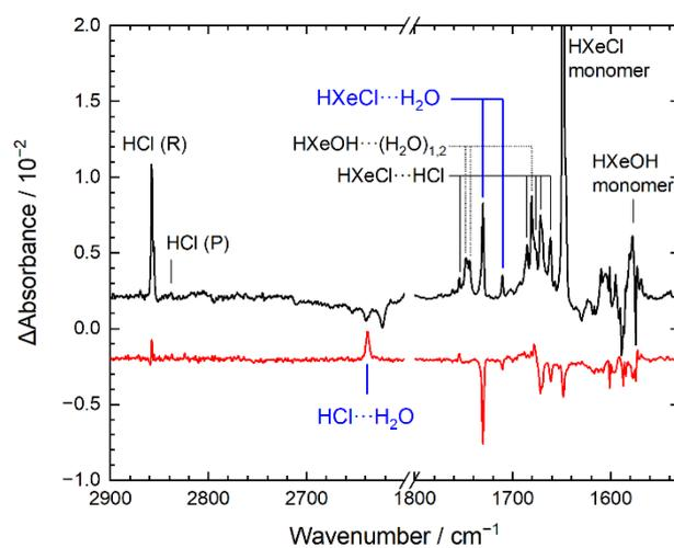
**Fig. 4.** Infrared difference spectra showing the results of (upper) annealing at 40 K of the photolyzed HCl/H<sub>2</sub>O/Xe matrix and (lower) subsequent annealing at 45 K. Prior to these experimental steps, the HCl/H<sub>2</sub>O/Xe matrix deposited at 40 K was photolyzed by 193 nm light. Spectra were measured at 3 K.
