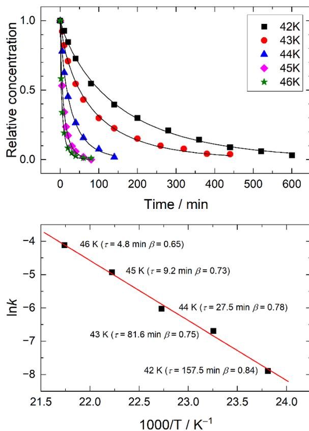
**Fig. 6.** Upper: Thermal decomposition of the HXeCl $\cdots$ HCl complex at temperatures 42–46 K. Solid lines represent the results of least-square fits with the stretched exponential function. Lower: Arrhenius plot of the decomposition. Parameters (decay time constant,  $\tau$ , and stretching exponent,  $\beta$ ) determined for each temperature are indicated. The solid line represents the simple linear regression.
