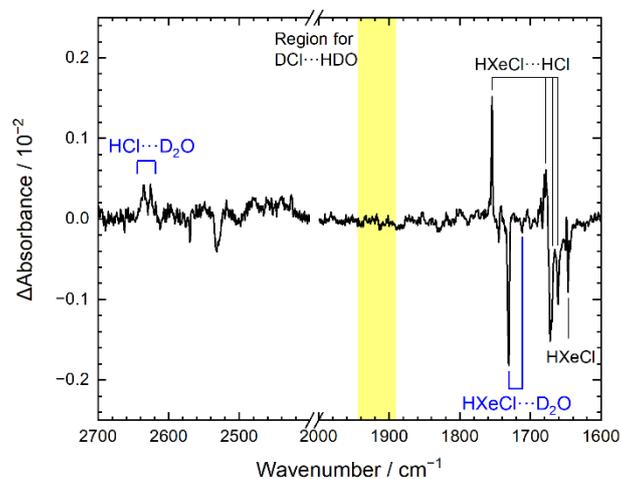
**Fig. 5.** Infrared difference spectrum of an HCl/D<sub>2</sub>O/Xe matrix showing the result of annealing at 45 K for 80 min. Before this experimental step, the HXeCl···D<sub>2</sub>O complex was produced by photolysis at 193 nm followed by annealing at 40 K for 80 min. The spectra were measured at 3 K. The absence of the DCl···HDO complex is indicated with a yellow rectangle.
