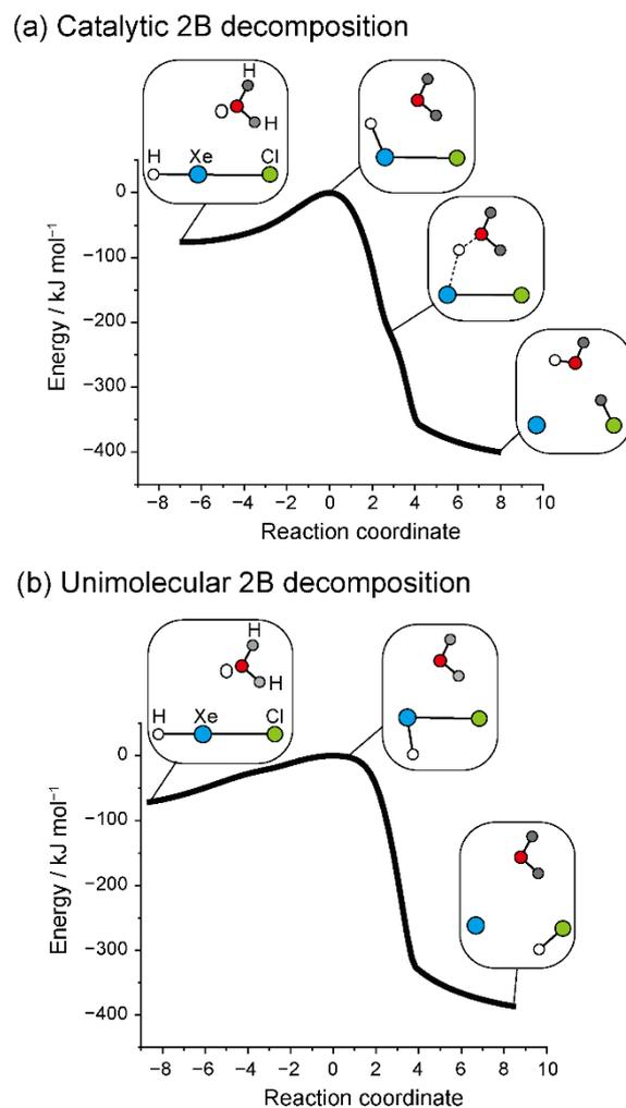
**Fig. 3.** Reaction paths along the intrinsic reaction coordinate for (a) catalytic 2B decomposition and (b) unimolecular 2B decomposition. Calculations were performed with the MP2/def2-TZVPPD method. Hydrogen atoms in the HXeCl and H<sub>2</sub>O moieties are shown in different colors (white and dark gray, respectively) so that the hydrogen exchange in the catalytic decomposition process is easily recognized.
